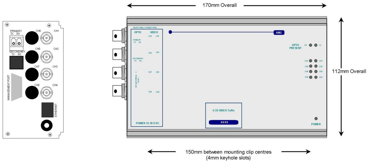
The **AMG4641T** is a standalone four channel video transmit unit designed to transmit 4 video signals over one Multimode fibre.
